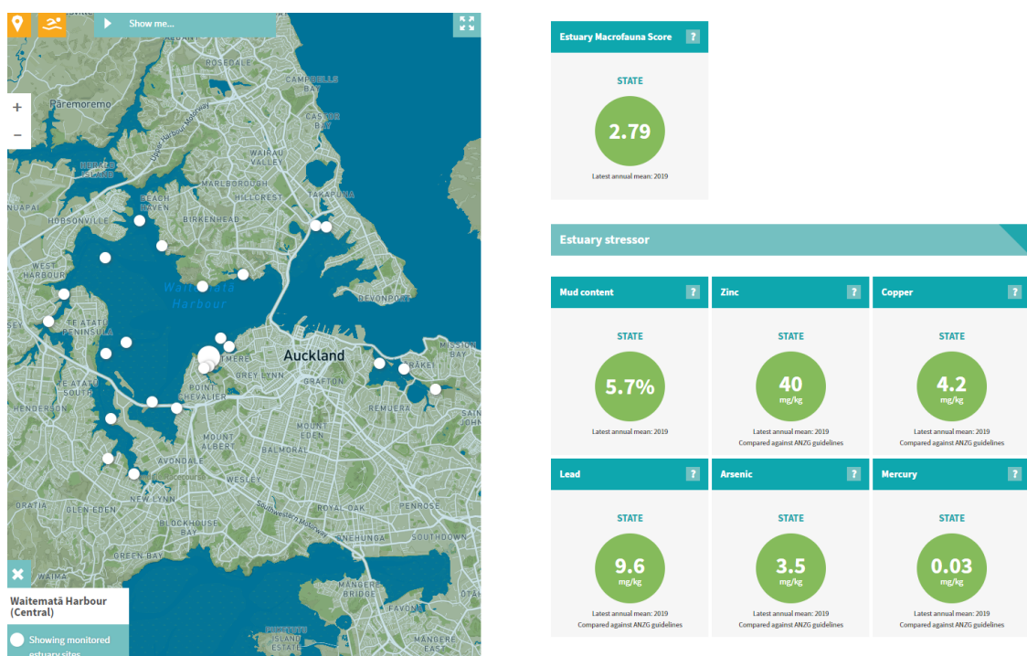
Figure 21 Example of estuarine stressor (heavy metal) monitoring from the LAWA website https://www.lawa.org.nz/explore-data/estuaries/ that could potentially be used as an indicator of shellfish edibility. This example is from the Meola monitoring site with data collected by Auckland Council (image captured 29 April 2024).
