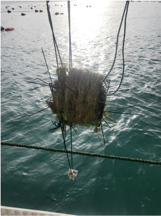
Figure 4 Photograph of a replicate of “fluffy” harakeke natural fibre rope wrapped around a plastic frame before being deployed on the mussel spat farm in Aotea Harbour.
