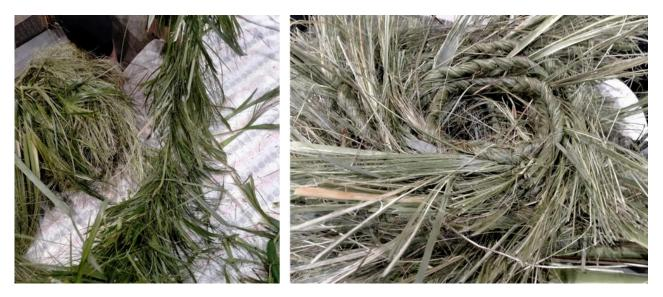
**Fig. 2.** Photographs of natural fibre ropes manufactured by plaiting techniques by iwi project partners, Ngāti Manuhiri (left – harakeke, right - tī kōuka) that were used for assessing fibre resistance to seawater.
