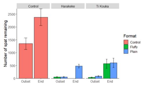
Fig. 3. Mean (± SE) number of spat attached per metre of experimental rope for plastic spat-catching rope (ie control) and two natural fibres (ie harakeke and tī kouka) prepared into two rope designs (ie fluffy and plain) after being at a spat-catching site for two months (ie outset) and after transfer to a coastal mussel farm.
